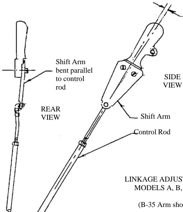
In the forward position the control rod centerline should be slightly to the rear of the shift arm centerline. This provides an "over center" toggle locking effect which prevents the gate from being forced into reverse. Slot the screw holes in the shift arm if necessary to allow reaching in this position. Adjust the length of the control rod so that the gate is forced solidly against the rubber pad in forward position.
