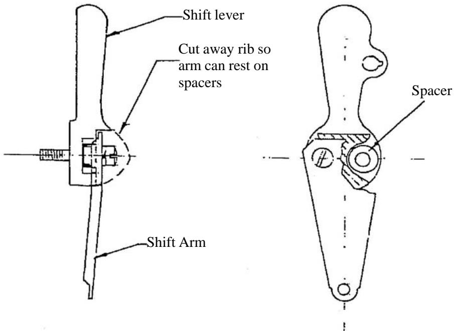
Modification to shift lever to receive B-35 Shift Arm and Spacers. Evinrude shift lever Part No. 278282 can be used without modification
